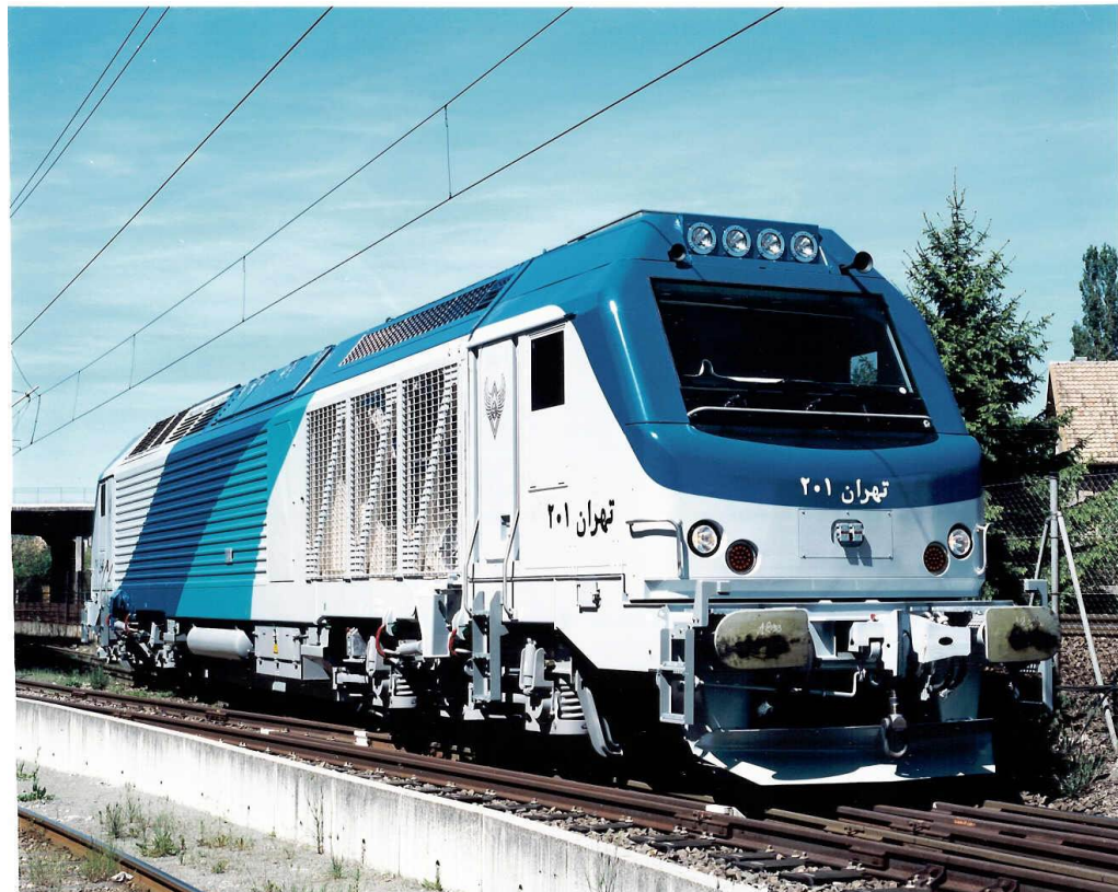
Main line Locomotive AD43C (Under Licence of Alstom)
